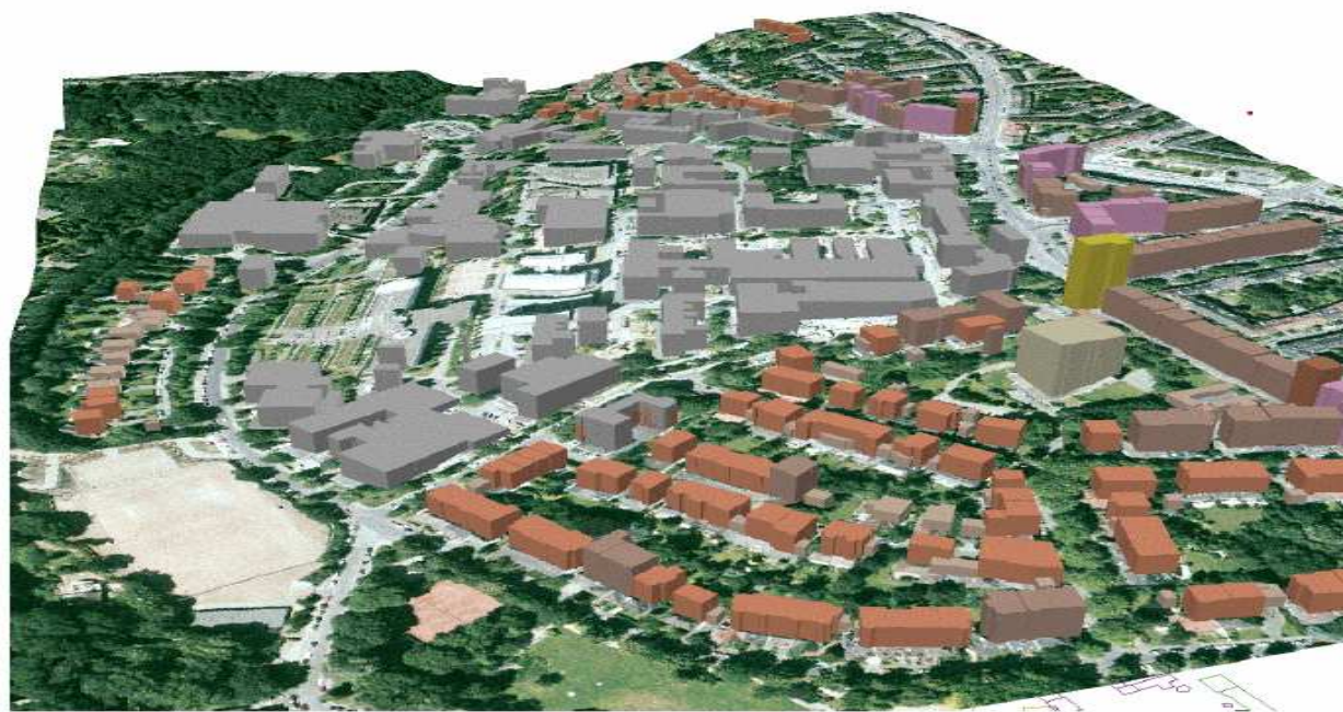
Figure 7.4.2a Animation for a building project in Essen NRW, LoD1 (Virtual Construction support ViCON), CAD Data + 10m grid terrain model + GeoTiff, ArcSecne, Output VRML for Navisworks, External Presentation and internal discussion.
